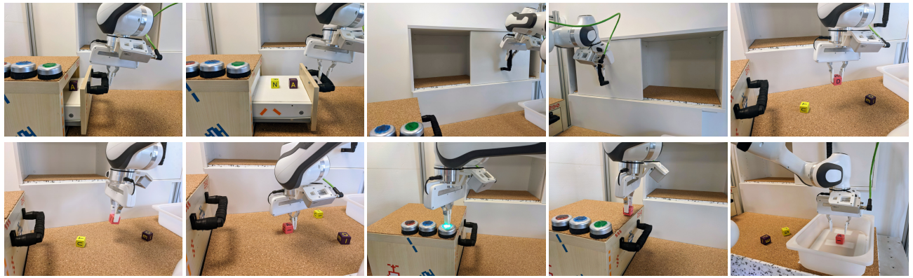
Figure 4. Real-world Manipulation Tasks. Examples shown from left to right are: closing the drawer, opening the drawer, moving the sliding door left, moving the sliding door right, lifting the block, rotating the block, pushing the block, turning the green LED on, placing the block on top of the drawer and placing the block in the container.
